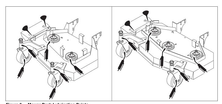
Figure 6. Mower Deck Lubrication Points
